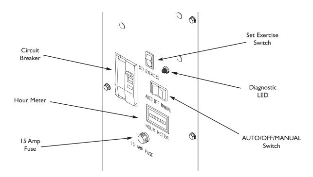
**15 Amp Fuse** — Protects the Backup Power System DC control circuits. If the fuse has 'blown' (melted open) or was removed, the engine cannot crank or start. Replace the fuse using only an identical BUS AGC 15A fuse.
